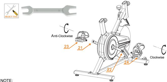
Right foot installation is clockwise, Left foot installation is counterclockwise.
